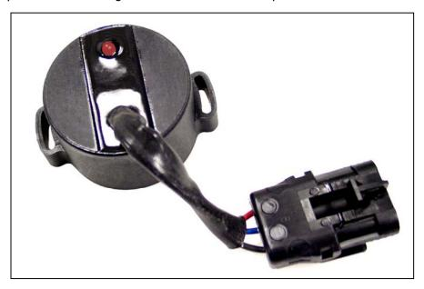
Since the slot can allow 50 degrees of rotation, we will only need to use half of the slot to make our 25 degree index adjustment. To attain the 25 degree offset, start by installing the sensor cap with the screws over to the side **EXACTLY AS SHOWN** in this illustration:
